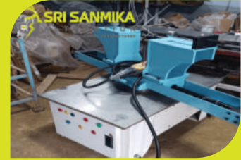
VALVE 360° Rotation fixture for testing
