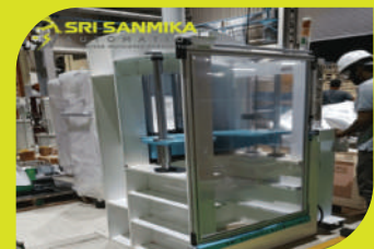
CUSTOMIZED HYDRAULIC PRESS FOR FRONT LOADING
